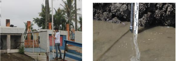
Figure 2 Sea Level Measurements taken with a bottom pressure record (BPR) AANDERAA and visual readings of the tidal staff taken at Praia Grande
