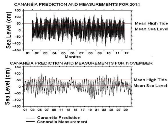
Figure 06. The upper part of the Figure shows the line of Mean High Tides (Sizyges) and Mean Sea Level Line for the entire year of 2014 and in the second part the corresponding month of November 1831, obtained by Retro-Prediction, with the actual data obtained by KALESTO from the Research Station of Cananea.
