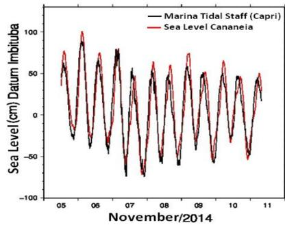
Fig 4 - Sea Level at PG and at Cananea Research Station, reduced to altitudes relative to the Imbituba datum. Note that the mean altitudes of both places are referred to equal to zero.
