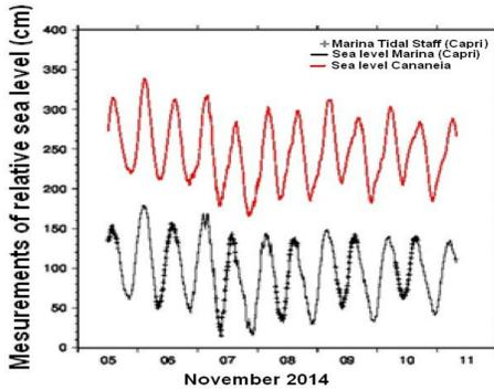
Figure 05 .Measurements taken at Marina Capri during days 05 to 11 of November of 2014, compared to similar measurements taken at Cananea (in red color). The crosses indicate the measurements taken by visual readings of the tidal staff. Mean High Water Tide (Sizyges) of 1831
