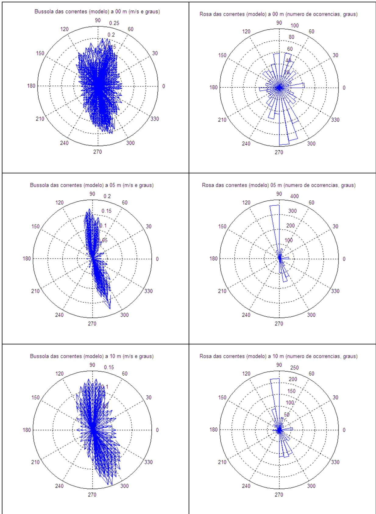
Fig. 9 - Currents compass and roses at the surface, 05 m and 10 m depth, computed by the hydrodynamic numerical model at the point of ADP measurements, in January / February 2010.
