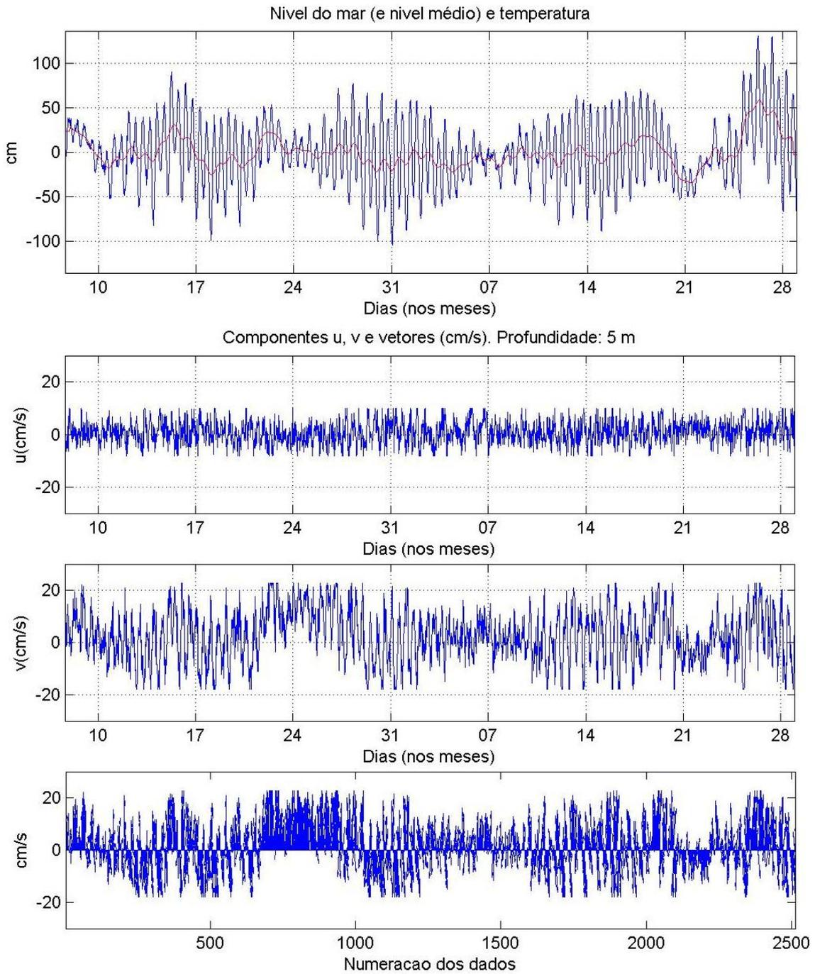
Fig. 5 - Time series of sea surface level (and mean sea level), EW and NS current components and current vectors at mid water, in the period from 16:30 GMT January 7 to 00:30 GMT March 01, 2010 - measured by Sontek Argonaut.
