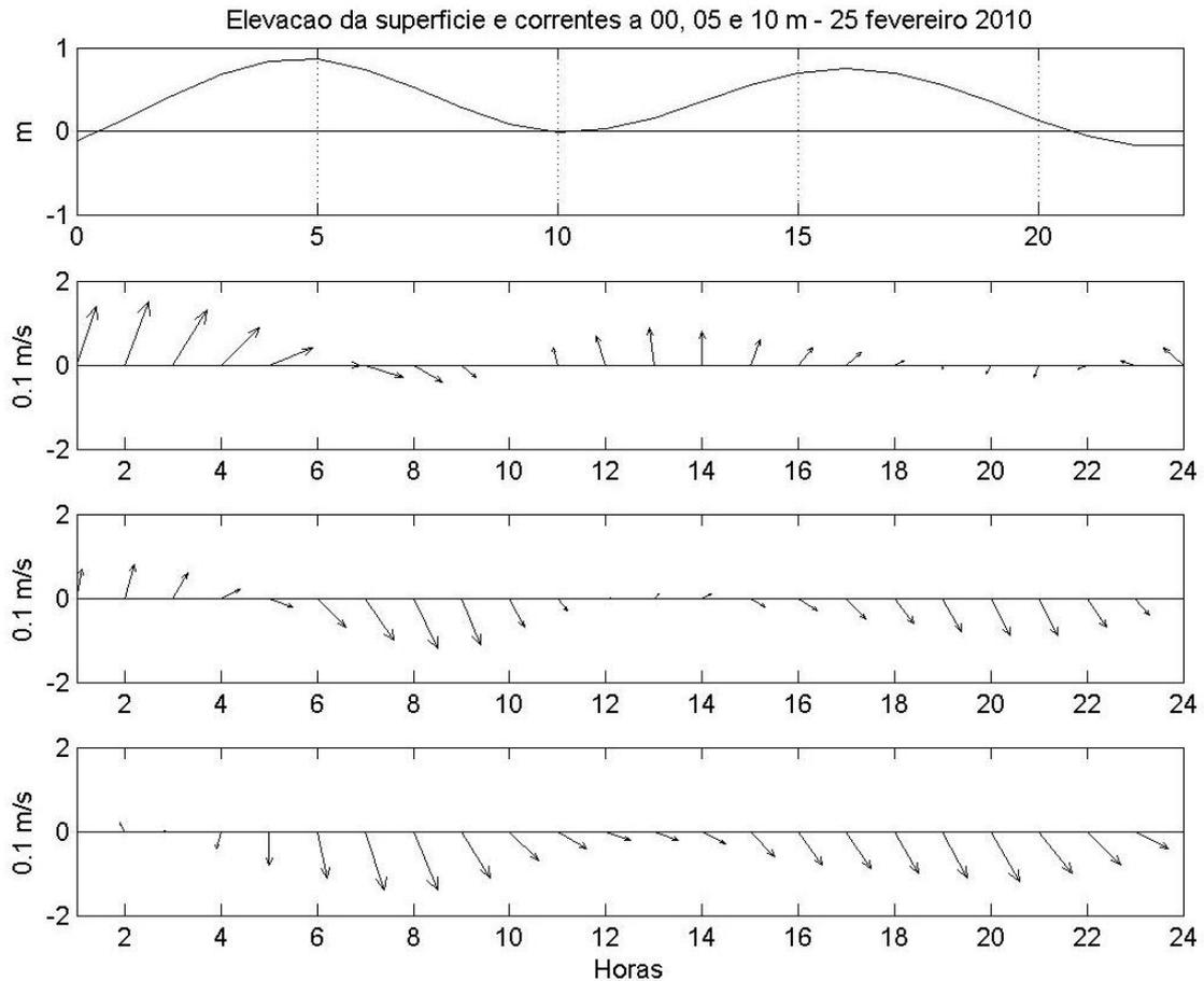
Fig. 10 - Sea surface level and sea currents at the surface (0 m), 5 m and 10 m depth, computed by the hydrodynamic model for the day 25 February, 2010, at the same position of the ADP measurements.
