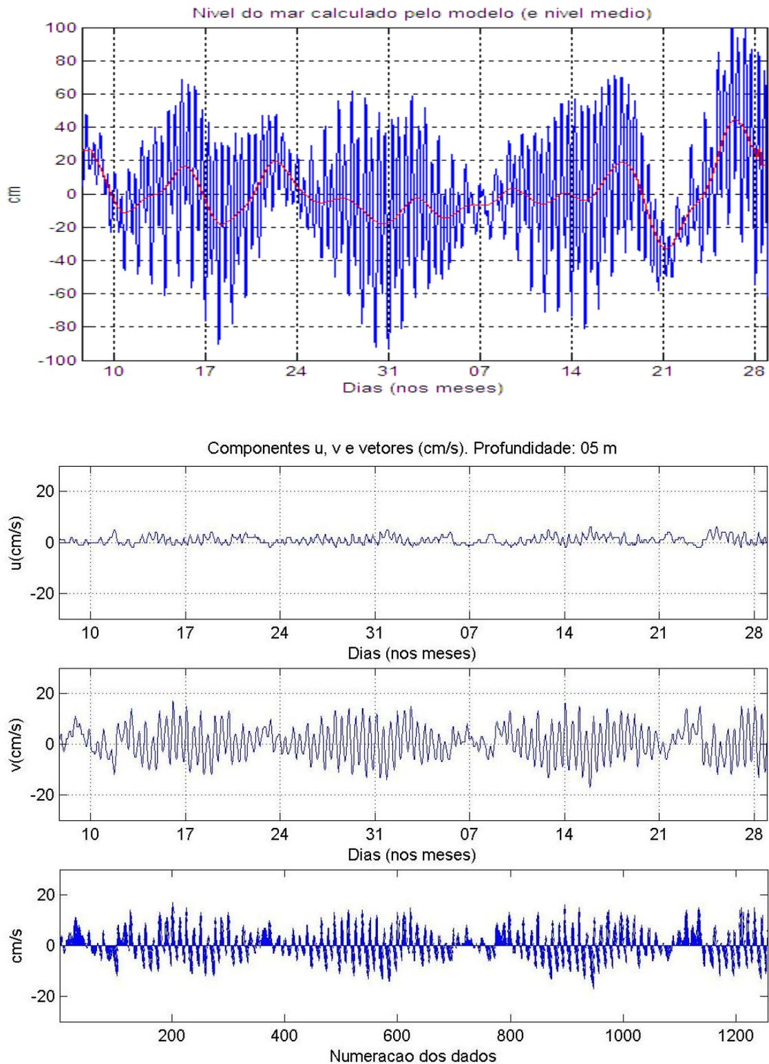
Fig. 8 - Time series of sea surface level (and mean sea level), EW and NS current components and current vectors at mid water in January / February 2010, calculated by the model, in the point of ADP measurements.
