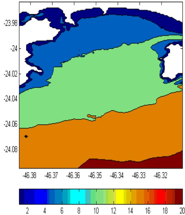
Fig. 1 - Bathymetry of the high resolution grid (in meters), centered in the Bay of Santos.
