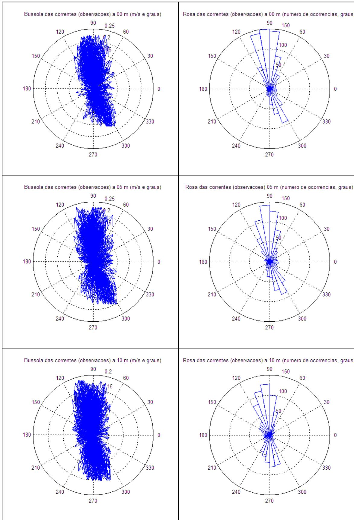
Fig. 6 – Currents compass and roses measured by the Sontek Argonaut in January / February 2010, considering the currents at the surface, 05 m and 10 m depth.
